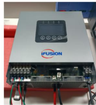
1 Boards: COM * 1 AC IN * 1, AC OUT1 * 1, AC OUT2 * 1, BAT * 1, PV * 1
